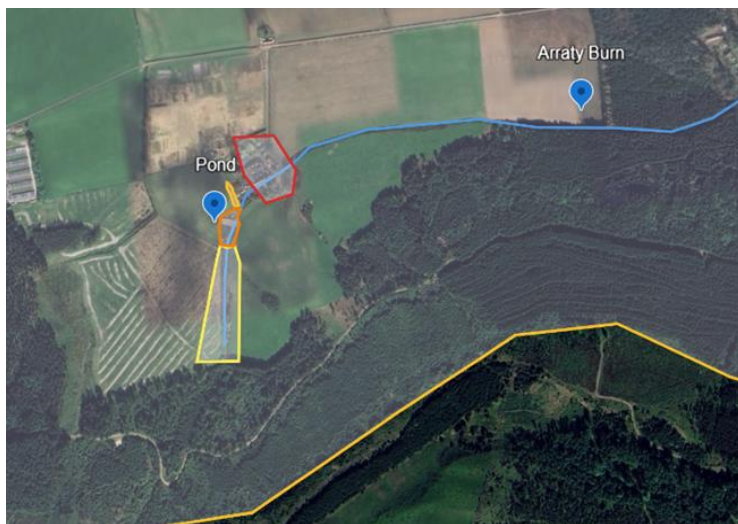
Figure 31: Constructed pond (orange) that leads to flooding of houses downstream (red). Options to reduce overflow (yellow) include leaky barriers and a sediment pond upstream of the pond, while overflow could be diverted to a fenced-off field margin. Map created using Google Earth (2025). Data attribution: AirbusData SIO, NOAA, U.S. Navy, NGA, GEBCO
