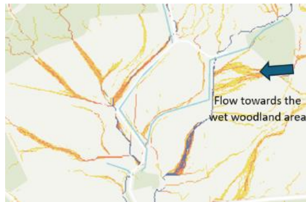
Figure 21: Flows towards wet woodland. Map created in ArcGIS Pro 3.5.0 (Esri Inc, 2022) using LiDAR data from the Scottish Government (2022) Remote Sensing Portal using a 2m digital elevation model, resampled to 4m grid resolution for flow accumulation analysis.
