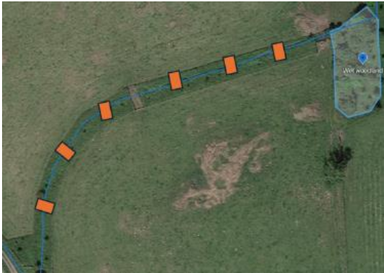
Figure 22: Potential placement of leaky dams (orange) to slow the flow downstream. Map created using Google Earth (2025). Data attribution: AirbusData SIO, NOAA, U.S. Navy, NGA, GEBCO
