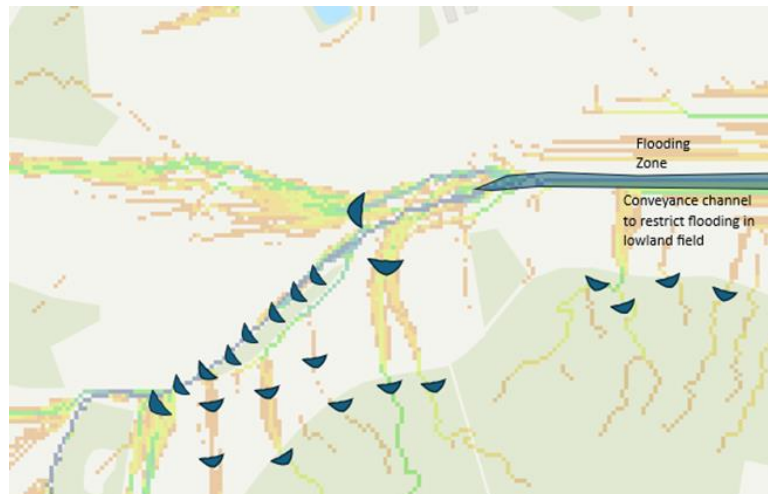
Figure 9: Overview of water management options for infield pathways. Map created in ArcGIS Pro 3.5.0 (Esri Inc, 2022) using LiDAR data from the Scottish Government (2022) Remote Sensing Portal using a 2m digital elevation model, resampled to 4m grid resolution for flow
